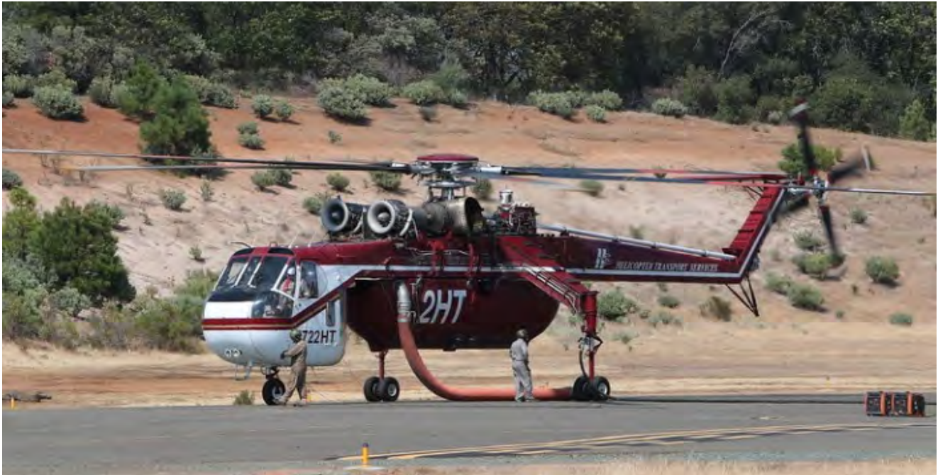
FIGURE 11: TYPE 1 HELITANKER WITH 2,400-GALLON TANK
