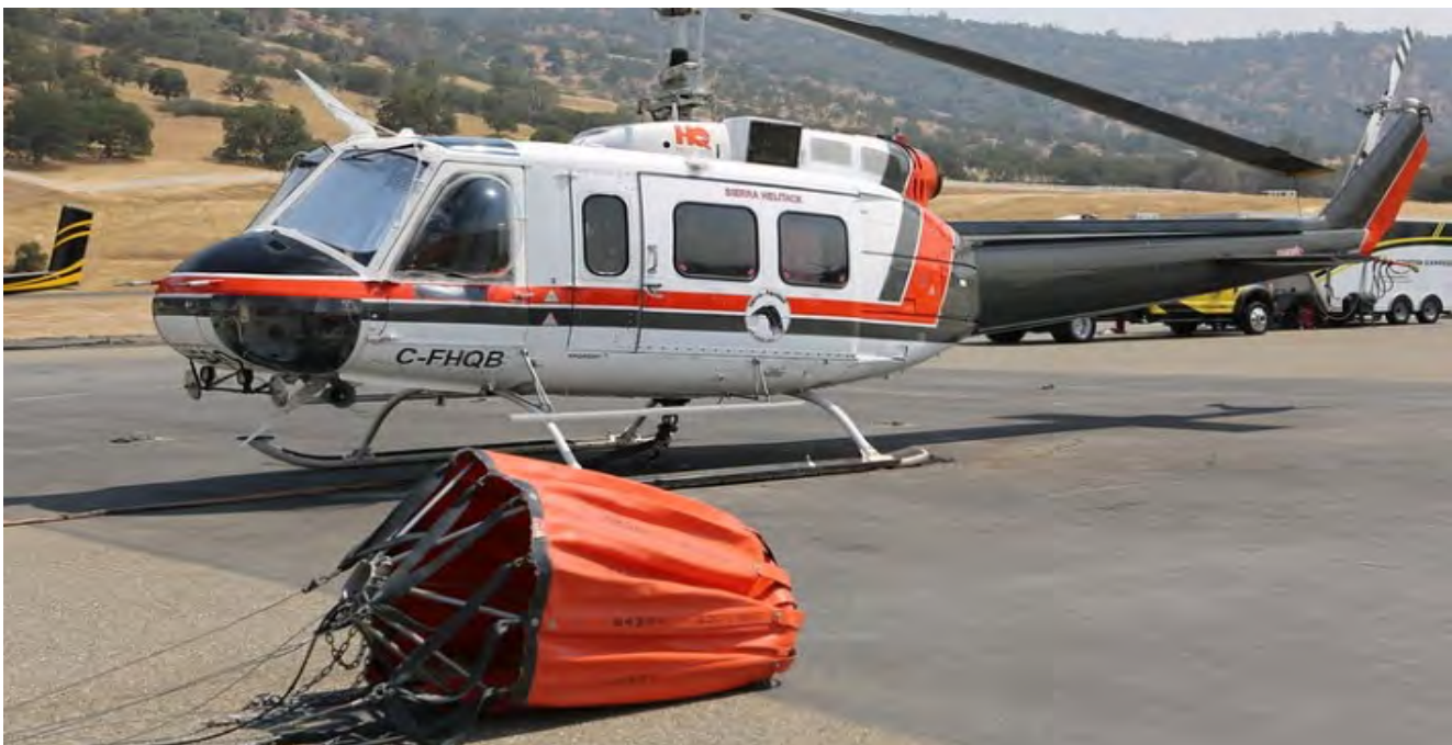
FIGURE 12: TYPE 2 WITH 360-GALLON BUCKET
