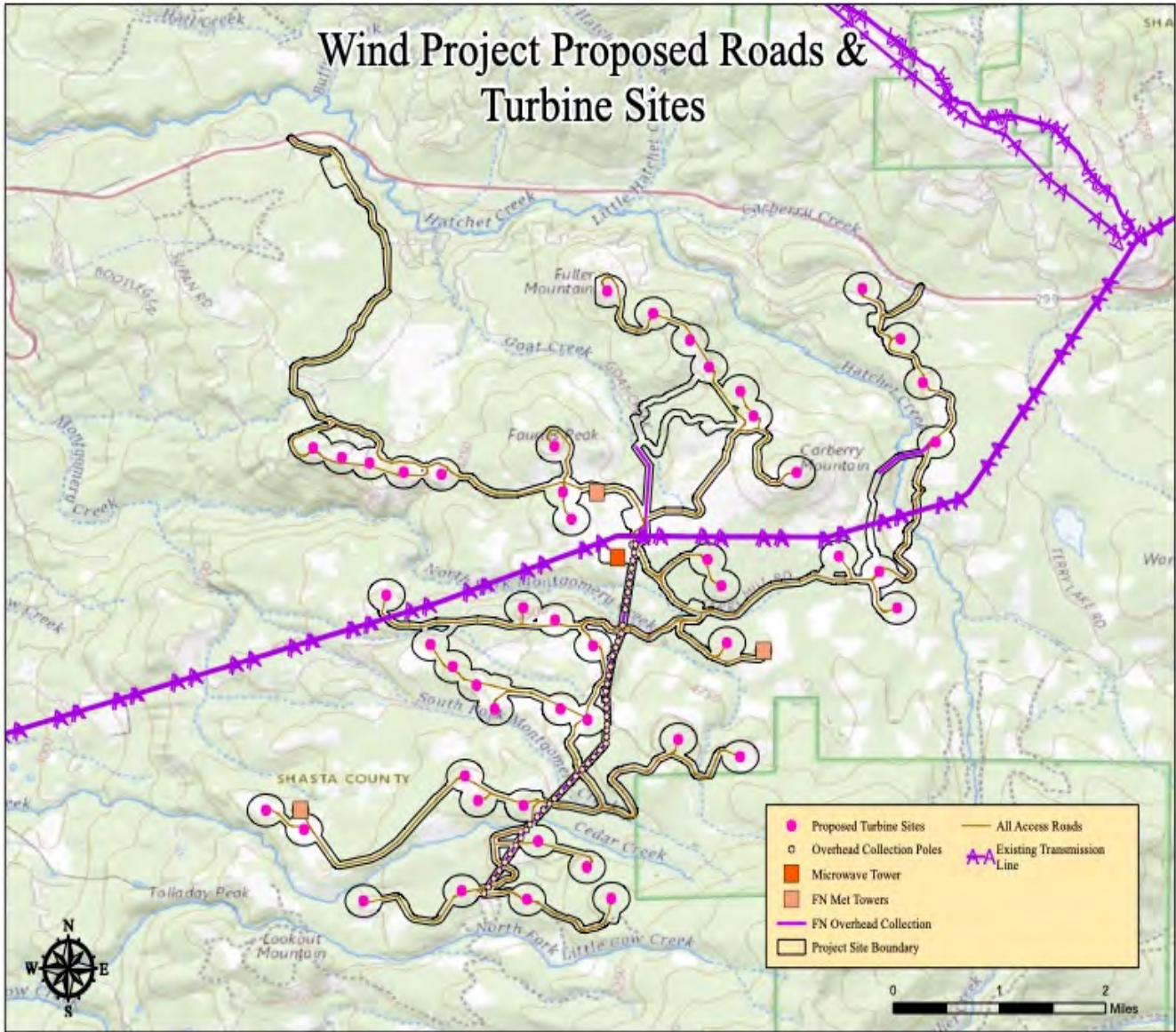
FIGURE 2: CIRCLES AROUND PROPOSED TURBINES REPRESENT THE REMOVAL OF 2.5-ACRES OF VEGETATION AROUND THE TURBINES; THE ROAD EDGES ARE SHOWN TO ILLUSTRATE THE SHADED FUEL BREAKS ALONG THE ROADWAYS.
