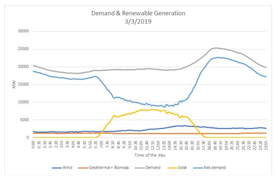
"Duck Curve" depicts system integration needs when there is excess generation on the system (the "duck's belly") and when extra "ramping" resources are needed in the evening as the sun goes down while customer demand is rising.
